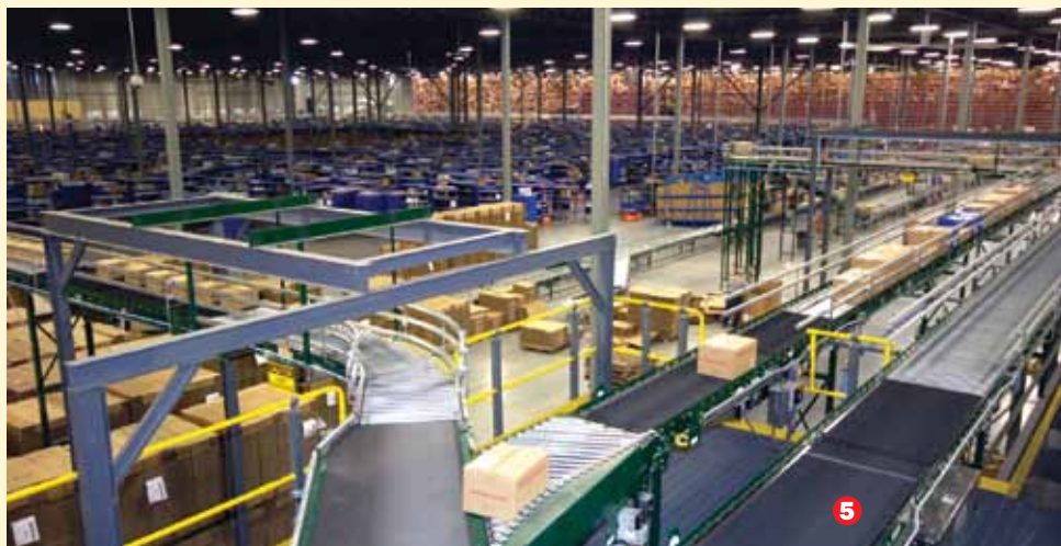
1. Picking instructions are delivered to a touchscreen. 2. Associates pick items from a portable module. 3. Picked items are placed on a portable module. 4. Mobile robots deliver the modules to the conveyor system (5) for induction. 6. Cartons are sorted to a packing station.
