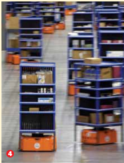
1. Picking instructions are delivered to a touchscreen. 2. Associates pick items from a portable module. 3. Picked items are placed on a portable module. 4. Mobile robots deliver the modules to the conveyor system (5) for induction. 6. Cartons are sorted to a packing station.
